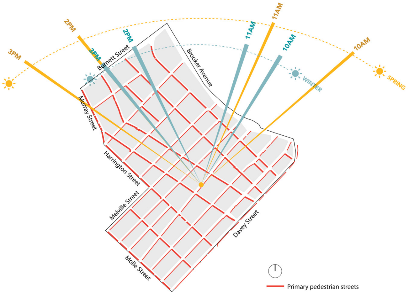
Sun angle plan for winter solstice and spring equinox
